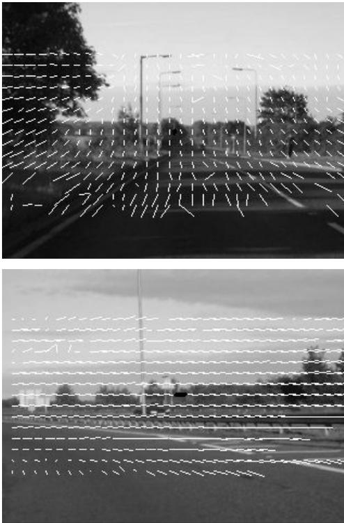
Figure 8. Optic flow on straight road (top) and while turning (bottom)
