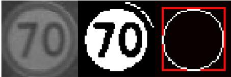
Figure 5: Removing red boundary from numerical-limit sign candidates
