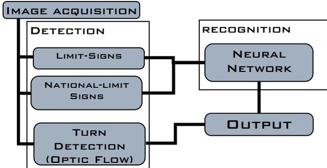
Figure 2. Structure of the algorithm
