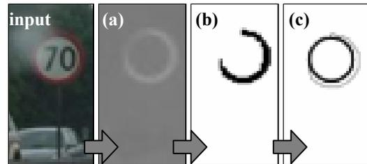
Figure 3: Steps of numerical-limit signs candidates generation algorithm
