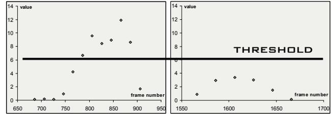
Figure 9. Mean optic flow over 15 frames. Turning (left) versus overtaking (right)
