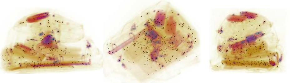
Figure 5: Keypoint locations for a typical complex baggage item
