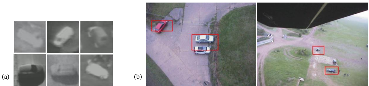
Figure 4. (a) Thermal imagery - signatures of cars; (b) Example detections of vehicles in optical imagery.
