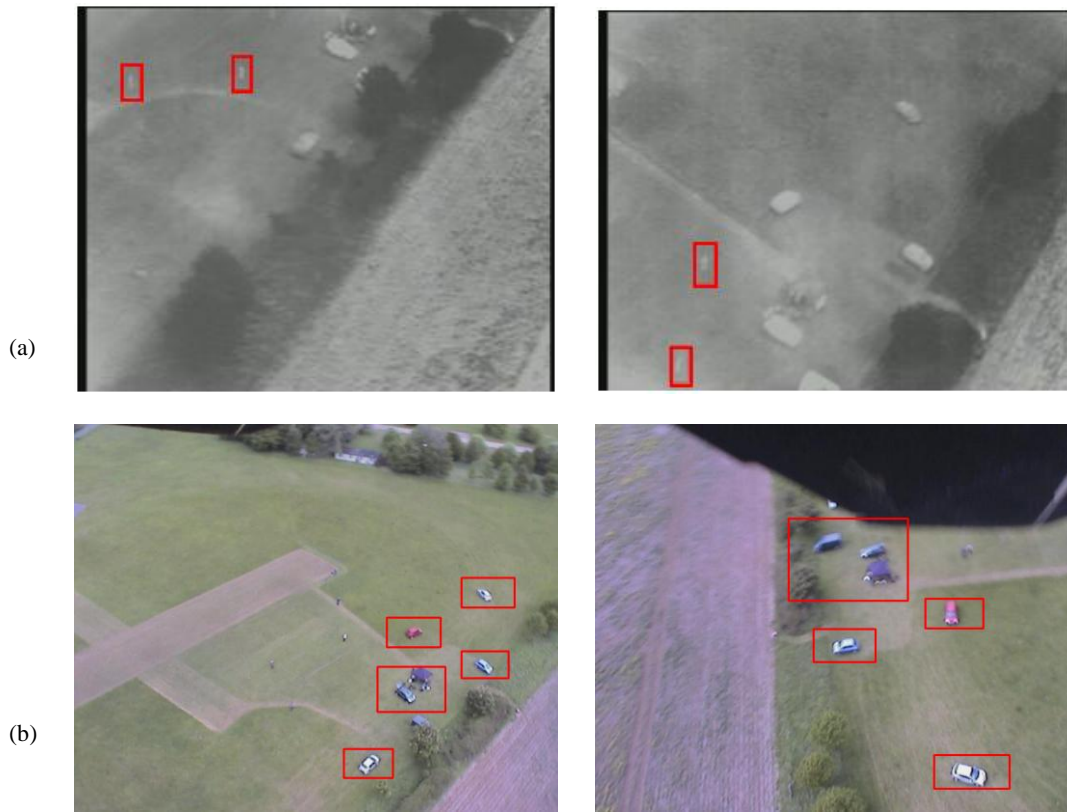
Figure 8. People detection results in thermal imagery (a) with optical images of the same scene with vehicle detections (b) (summer conditions).
