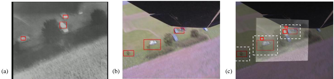
Figure 7. (a) Identified thermal signatures; (b) Vehicle detections; (c) Fused detections from thermal and optical images.
