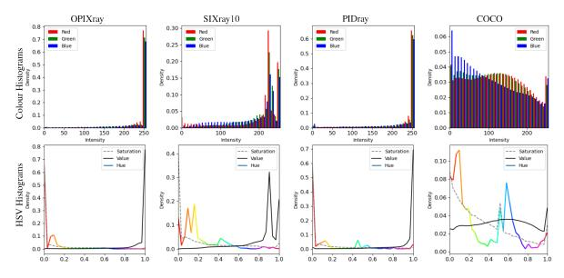
Figure 3. RGB and HSV histograms for X-Ray datasets: OPIXray [40], SIXray10 [26] and PIDray [41]; compared with COCO dataset [21].
