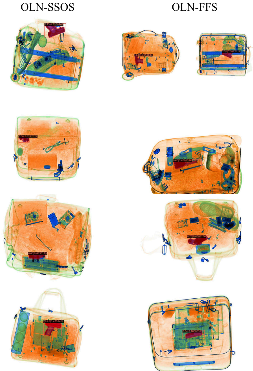
Fig. 21: Qualitative results for DBF6 (Mask). No baseline is presented since there is no baseline for instance segmentation. In all of the examples, it can be noted that both methodologies get the correct segmentation mask, with the exception of the missed gun for OLN-SSOS in the second row.
