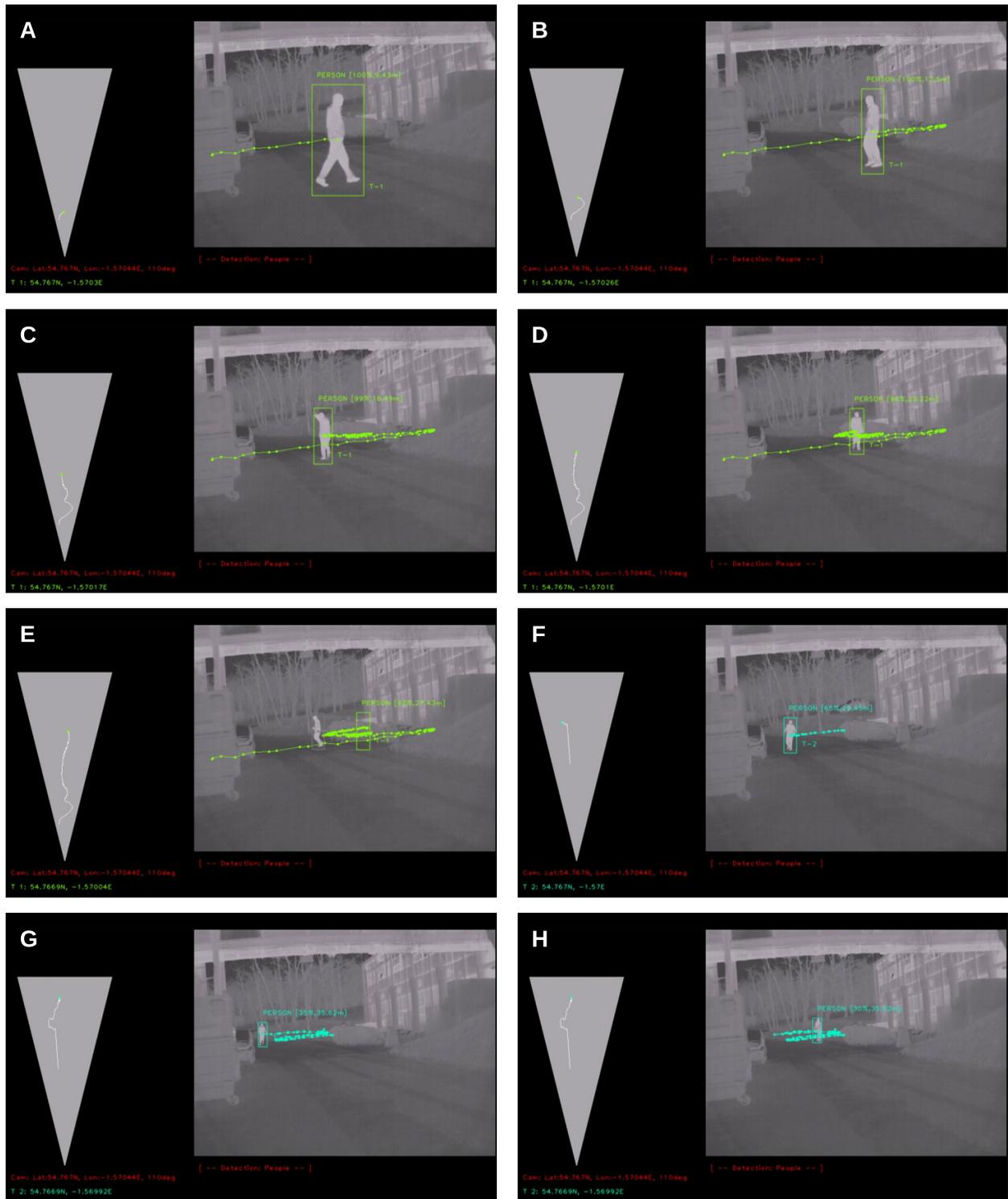
Figure 8. An example of real-time pedestrian detection and tracking in infrared imagery (right) with associated geo-referenced 3D track (left).
