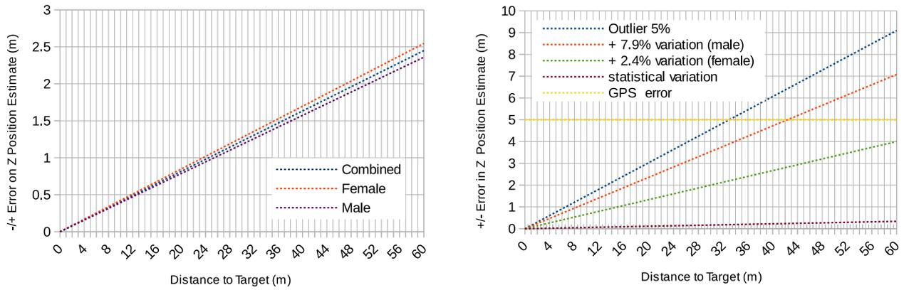
Figure 3. Position error in  $Z$  (distance to target) attributable to variation in height for standard deviation of 7cm (left) and for cases of additional height variation due to genetics and age differences (right)
