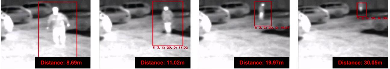
Figure 2. Photogrammetry facilitates the approximate recovery of a camera to target distance for an example target (person) without any need for additional (active) range sensing [2]
