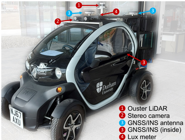
Figure 2: Test vehicle (Renault Twizy): equipped with a long range stereo camera, a LiDAR, a lux meter and a combined GNSS/INS inertial navigation system.
