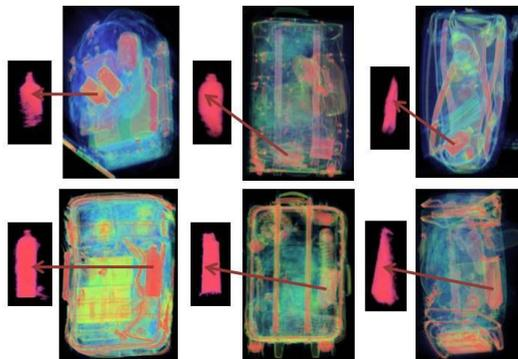
**Fig. 3.** Examples of detection results (bottles classified correctly) obtained by our detector.
