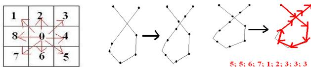
Figure 1: Definition of direction code, interpolation of laser pointer track and final gesture chain code
