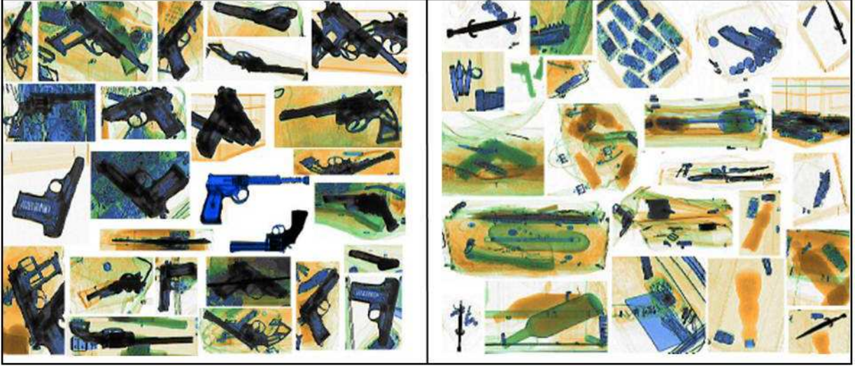
Fig. 3. Training data examples. Positive instances (left) showing firearms of various sizes, shapes, orientations etc. Negative instances (right) showing a variety of clutter items.
