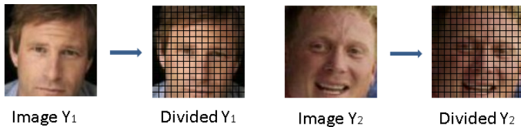
Figure 1: Face images are divided into I blocks. In this case, the input image is first resized to 120 \times 120 pixels, next divided into 15 \times 15 blocks. Size of each block is 8 \times 8 pixels, where I = 225 .
