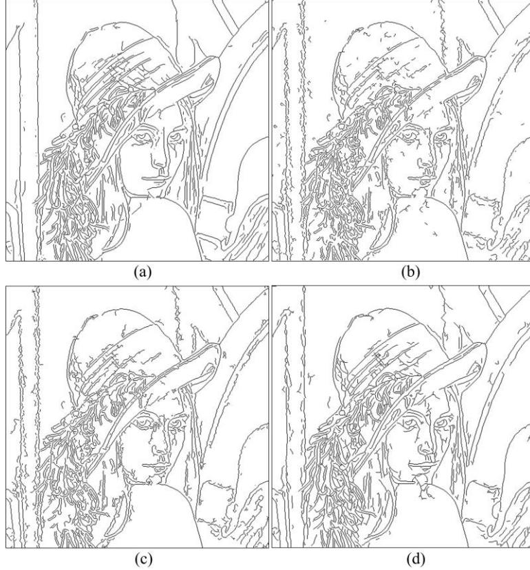
Fig.12. Visual comparison of the three detectors at  $\varepsilon_w = 15$ : (a) the ideal edge map; (b) edge map by Canny detector; (c) edge map by IAGKs detector; (d) edge map by the proposed detector.
